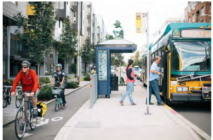
Cyclists riding in a protected bicycle lane beside a 'floating' bus stop in Seattle.
