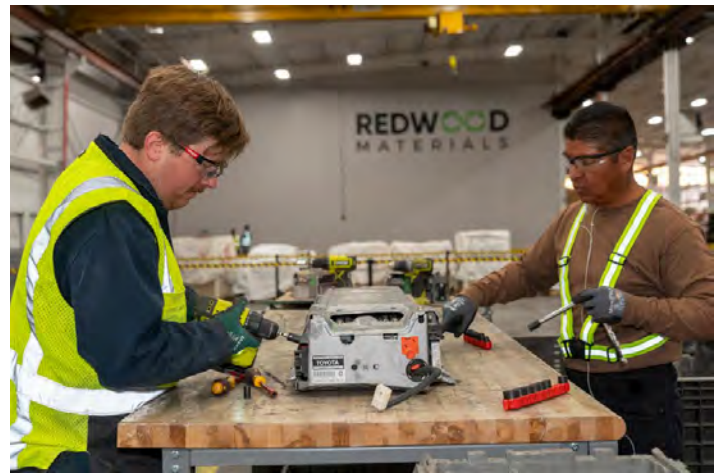
Workers disassembling an electric vehicle battery at Redwood Materials in Carson City, Nevada.
